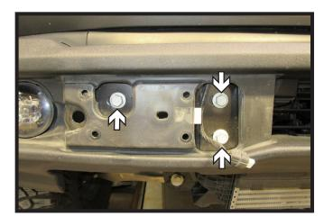
2. Using a 15MM socket, remove the three (3) bolts from the bumper. Do this on both sides of the vehicle.
