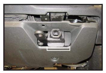
14. Hold the skid plate as close to its original position, mark and trim the skip plate around the convenience links and attachment tabs.
