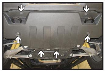
Using a 15MM socket, remove the six (6) bolts from the skid plate. Remove the skid plate and set aside to be reinstalled later.
