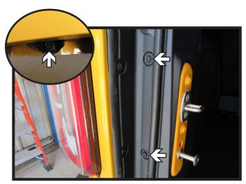
Using a 10MM socket, remove the three
