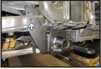
9. Using a 1/2" drill bit, drill the one (1) hole in the frame using the baseplate as a template. Do this on both sides of the vehicle.
