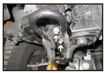
Using a 15MM socket, remove the two (2) bolts attaching the tow hook/housing to the vehicle. Remove the tow hook/housing and set aside, it will not be reinstalled. Do this on both sides of the vehicle.
