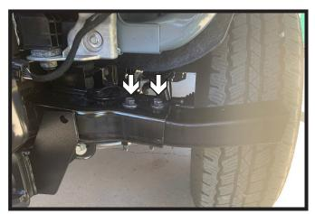
8. Vehicles with Frame Extension: Using a 15MM socket remove the two (2) bolts from the frame extension. Remove extension piece and set aside to be reinstalled later. Do this on both sides of the vehicle.
