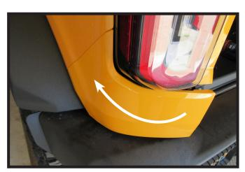
Carefully unsnap and remove plastic piece below tail light. Do this on both sides of the vehicle.
