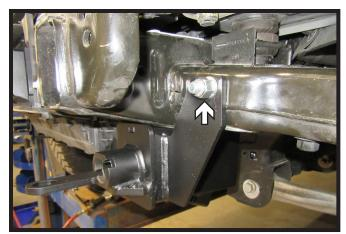
Using a 3/4" socket and wrench, install the one (1) 1/2" bolt with lock washer and nylon lock nut. Do this on both sides of the vehicle.
