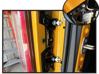
4. Using an 8MM socket, remove the two (2) bolts (white) and using a 10MM socket remove the one (1) bolt (gray, inset) attaching the tail light housing to the frame. Remove the tail light housing and install tail light wiring kit per kit instructions. Do this on both sides of the vehicle
