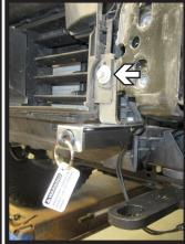
13. **Optional Breakaway**: Slide the breakaway bracket behind plastic piece and reinstall the existing bolt.
